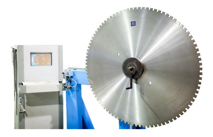
Asahi supplies new Diamond Excavator Blades to suit production saws and excavators ranging from 600mm through to 3,000mm
