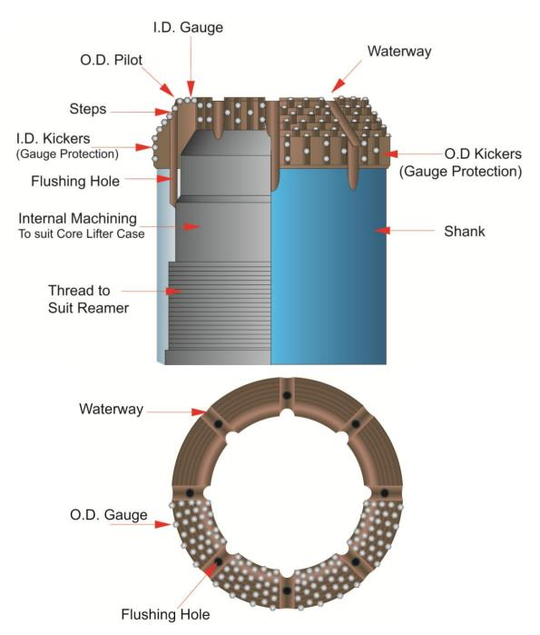
Drilling with Surface Set Bits generally continues until a substantial increase in required Bit weight indicates that the Diamonds have become "blunt" or broken, requiring the Bit to be pulled and either discarded or returned to the manufacturer for salvage.
