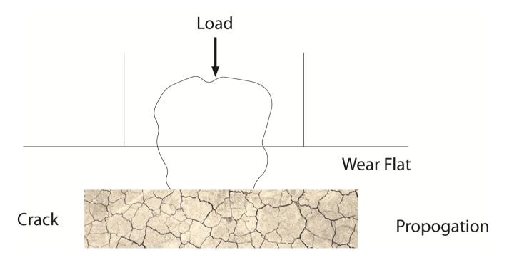
The performance of the Diamond is directly related to the wear flat area generated on the Diamond face.
