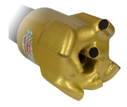
Polycrystalline Diamond (PCD) Bits have a purpose designed cast matrix head with 13.3mm round PCD inserts fixed in a cutting pattern. Non-CORE BITS are used for open hole drilling.
