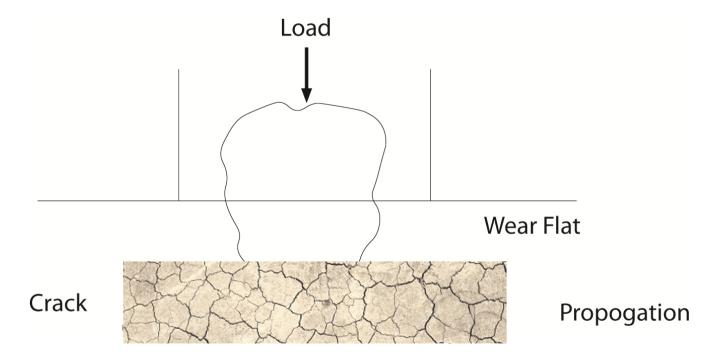
The performance of the Diamond is directly related to the wear flat area generated on the Diamond face.
