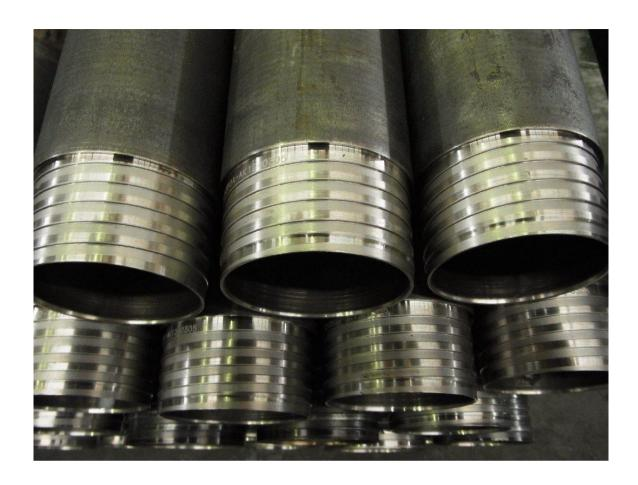
Wireline Drill Rods when used in conjunction with W/L Core Barrels allow the core to be retrieved through the Rods without removing the core barrel from the hole.
